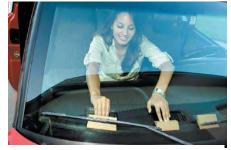
Insert cardboard wedges between your Coverlay dash cover and your windshield to create pressure on the dash cover edge against the window.
