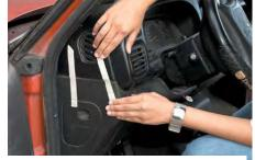
Use masking tape around edges of the dash cover to hold in place while silicone cures (approximately 6-8 hours). Once it has cured, remove tape and cardboard.
