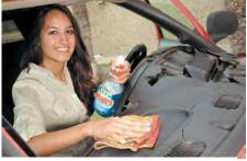
Clean your existing dash and the underside of your new Coverlay dash cover with an ammonia-based cleaner such as Windex®.
