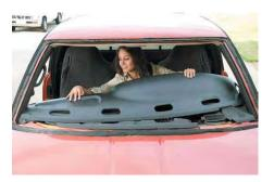
Test fit your new Coverlay dash cover. Minor adjustments sometimes are needed; use a utility knife or sandpaper. The dash cover should fit snugly over the entire dash. Practice putting it in place before moving to the next step.
